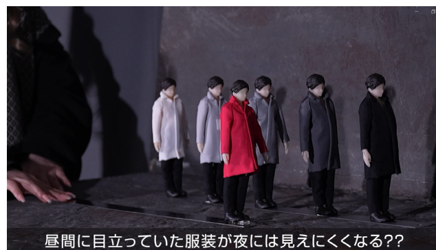
Visibility evaluation experiment of chromatic colors of pedestrian clothing using character figures and an actual car
