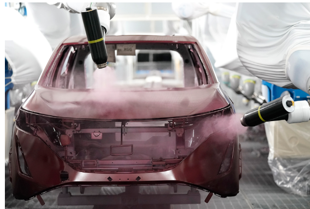
CO 2 emissions have been reduced by simultaneously painting the body and bumpers using a new technology and consolidating them into one process (right) and drying at a low temperature (85°C) instead of the conventional two-step process (left).
